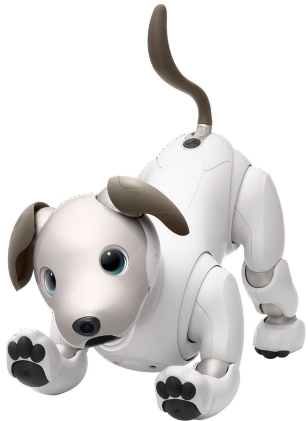
Fig. 1 aibo. Specification. Product name: aibo, model number: ERS-1000, processor: 64 bit quad-core CPU, display: 2 OLEDs (eyes), sound: speaker, 4 microphones, camera: 2 cameras (front camera, SLAM camera), communications: mobile network communication feature (data transmission) LTE, Wi-Fi IEEE 802.11 b/g/n (2.4 GHz), outside dimensions: approx. 180×293×305 mm, weight: approx. 2.2 kg, power consumption approx. 14 W, battery duration: approx. 2 h, recharge time: 3 h
